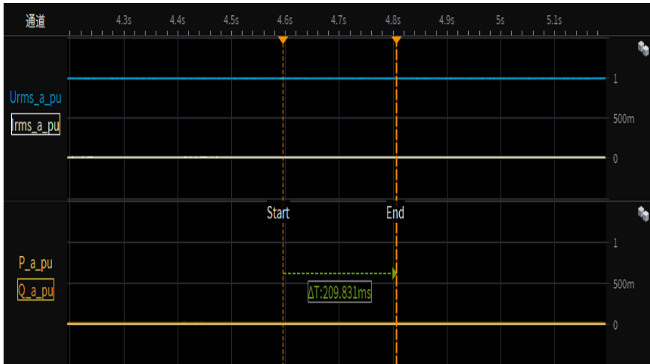
Test 5-1.1 Depth of fault phase: 0.1p.u.,LV two-phase-asymmetrical (type D),20% load Test overview(voltage,current,active and reactive power)
